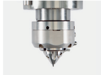
SP12 • High precision quick change automatic feeding collet – Runout/tilt adjustment – Internal high pressure flushing – Diameter range \varnothing 0.05 to \varnothing 1.5 \text{ mm} – Up to \varnothing 0.99 it fits to clamping range of 0.04 mm
