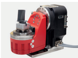
SX-Rotary A/B axis • High precision A/B axis – A rotary axis \pm 115^\circ – B rotation axis 360^\circ – Direct axis measurement – Designed for 3R or EROWA chuck – Resolution 0.0001 degrees – Workpiece holder internal flushing
