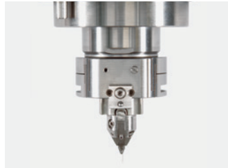
SP06 • High precision automatic electrode feeding collet – Runout adjustment – Internal high pressure flushing – Diameter range \varnothing 0.05 to \varnothing 1.5 \text{ mm} – Up to \varnothing 0.99 it fits to clamping range of 0.04 mm
