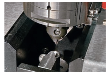
SX-Laser measuring • Laser for electrode diameter/profile measuring for SX-Arianne – Resolution of 0.10 \mu\text{m} – Minimum measurement of 0.005 \text{ mm}
