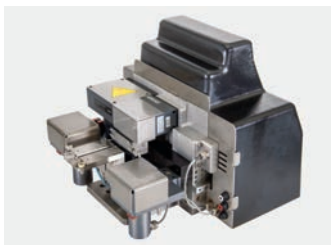
SX-Arianne • Wire Dress unit – Designed to produce micro-electrodes for micro-holes and micro-forms down to \varnothing 10 \mu\text{m} – Wire \varnothing 0.10 and 0.20 \text{ mm}
