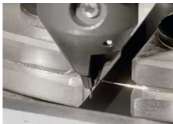
SX-Arianne • Wire Dress unit – Designed to produce micro-electrodes for micro-holes and micro-forms down to \varnothing 10 \mu\text{m} – Wire \varnothing 0.10 and 0.20 \text{ mm}
